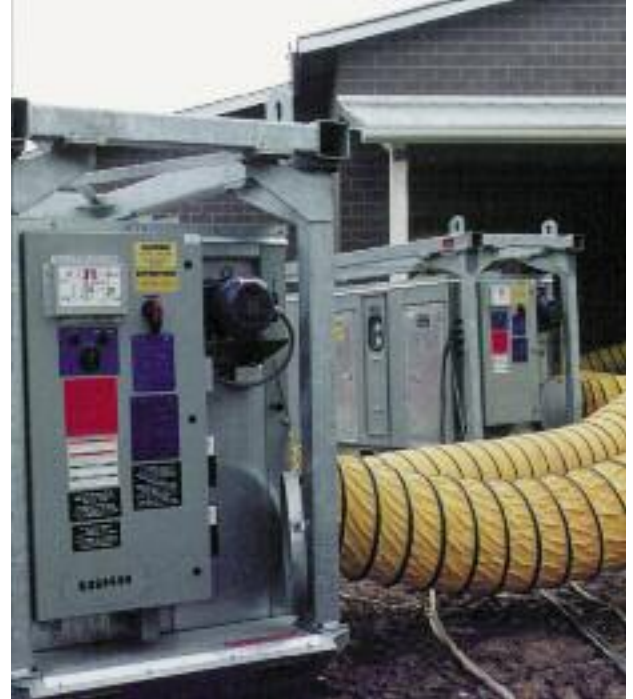
A MS-6000/5000 pulls moisture from ambient air.
