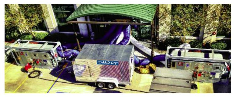
Skid-mounted - MS-6000/5000 with 18,000 SCFM trailer-mounted advanced filtration system.
