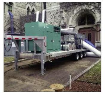
Trailer-mounted - MS-6000/5000 with heat recovery.
